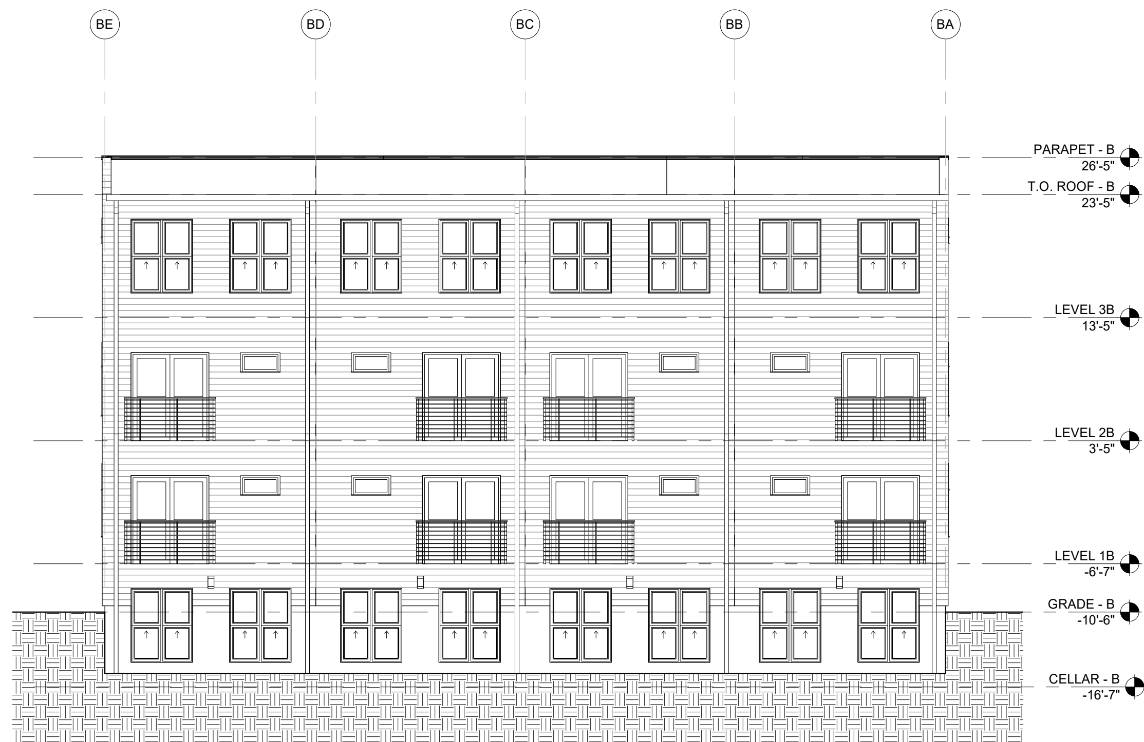
BUILDING B - NORTH ELEVATION 2 1/8" = 1'-0" A401
